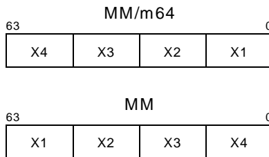
Figure 4-8 pshuf Instruction Example
