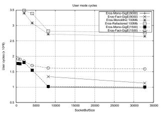
Figure 9: User cycles per 10,000 packets consumed during ttcp. Data for GigE(9000) for socketbuf lengths less than 8192 have been omitted to avoid graph compression. Measurements for smaller socket buffer sizes for the Gigabit (9000 mtu) case are limited by Linux transmit performance.
