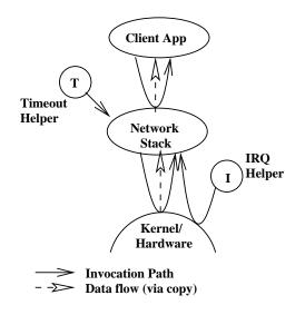
Figure 1: The EROS monolithic network subsystem
