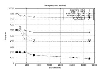
Figure 8: IRQs per 10,000 packets serviced during ttcp.
