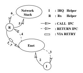
Figure 5: The various IPC invocations in the Rx data path. The numbers show the sequence of events.
