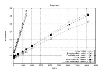
Figure 6: Ping times for the various stacks
