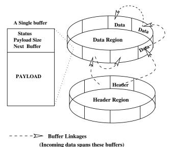
Figure 3: Receive ring buffers. The incoming data packet is scattered into header and client data and stored into appropriate ring buffers by the enet
